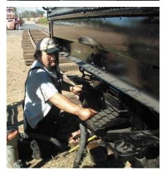
on the tender. Each "journal" box was jacked up, two large plates were removed, cotton waste that held the oil was pulled, bearings were lightly sanded, then everything was cleaned, oiled, and put back in place. The cotton waste was placed in gym socks that were soaked in journal box oil and then set under the bearings. Consequently, project coordinator Bill Aiken now has his personal gym socks as part of this historical display.
