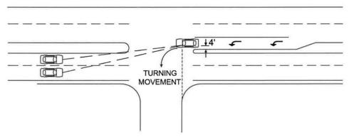
Sight Distance is based on a 3.5 foot height at the location of the driver and a 4.25 foot object height in the center of the approaching lane of the major road. The left turn driver measurement is taken 4 feet from the left edge of the turn lane at the projected edge of the curb return (as shown above). If the major road is a multi-lane road, the controlling measurement for sight distance shall be based on the approach lane that is the worst case scenario.
