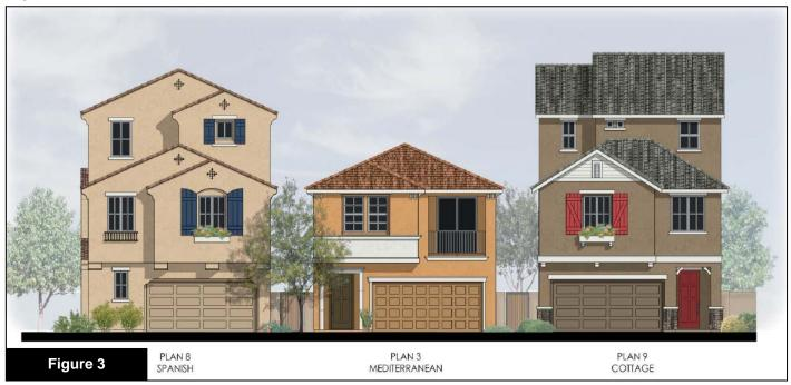
The roof elements are comprised of a combination of hip and gable elements. Various roof tile materials, colors and tones, compatible with the overall building color palette, will be utilized throughout the project to provide additional variation between buildings. The proposed building forms, colors, and materials meet the intent of the Community Design Guidelines.
